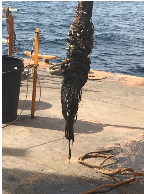
An end of one of the severed American Transmission Co. cables April 26, 2018. | ATC
